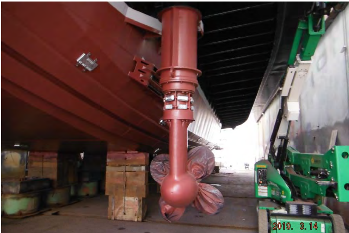
Photo No. 2 No. 1 end Z-drive Unit
