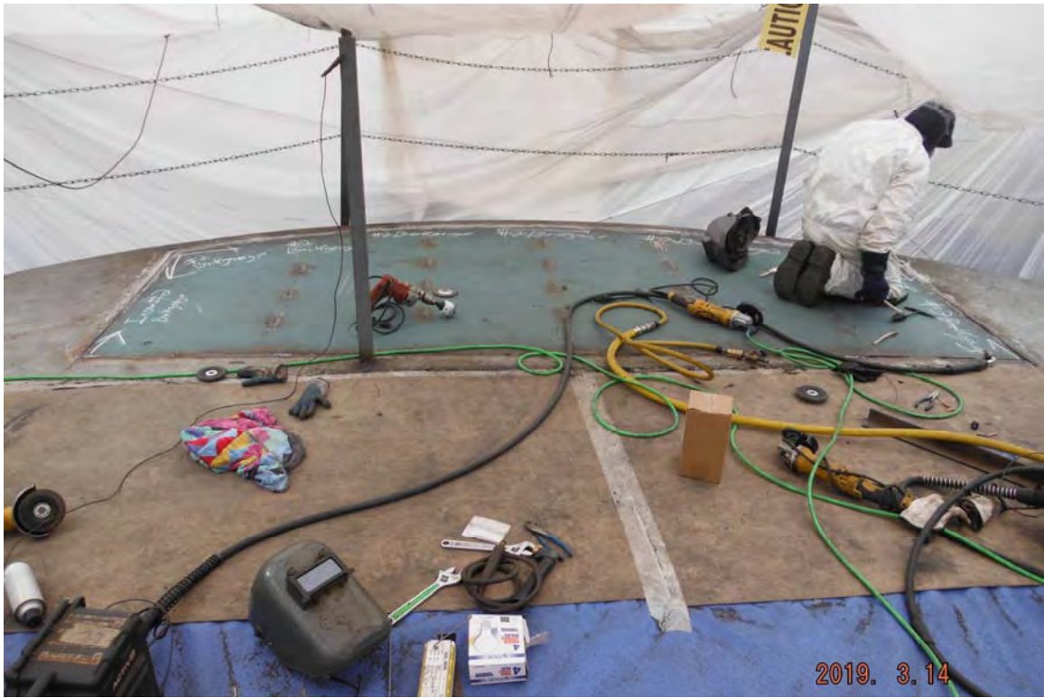
Photo No. 11 Main deck apron showing new insert
